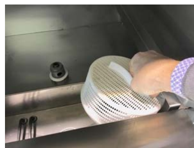
Remove the pump filter
