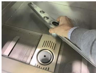
Replace the lower washing arm
