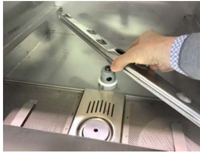
Remove the washing lower arm
