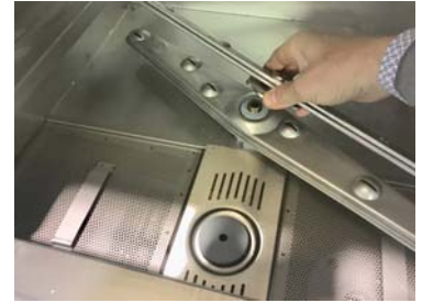
Replace the lower rinse arm
