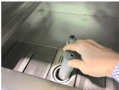
Remove the overflow pipe
