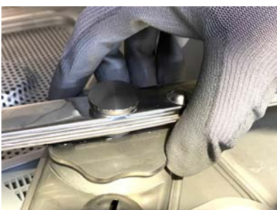
ATTENTION! Daily assemble the lower rinse arms by working on the „big“ ring nut, like in the picture.
