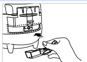
⑤ Insert the drain dish firmly by pressing it in direction of the arrow.
