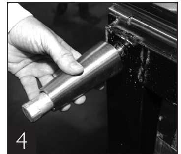
4 Thread leg into cabinet bottom frame rail.
