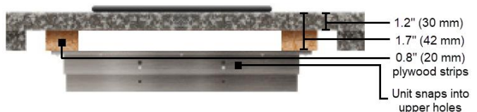
Figure 4-3: Stone Countertop 1.2" (30 mm) with Plywood Strips
