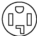
4-wire receptacle (14-30R)
