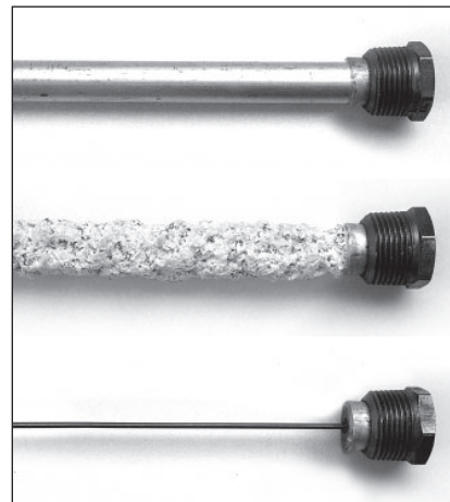
Figure 38: Anode rods from new (top) to partially depleted (middle) to fully depleted stage (bottom).
