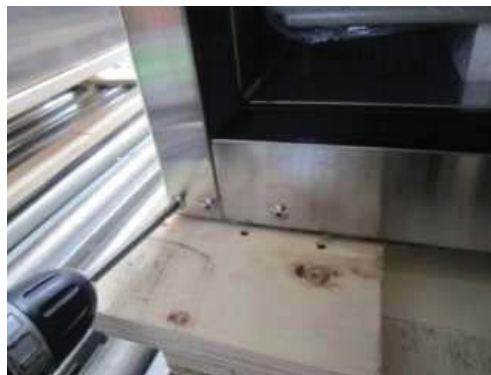
C-2. Disassemble bottom hinge (left).
