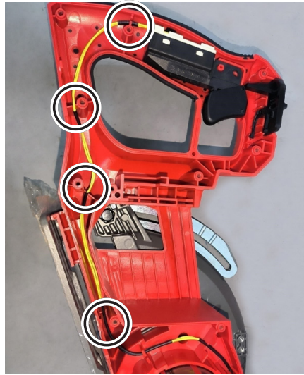
2) Press the switch wire into the housing traps and grooves.
