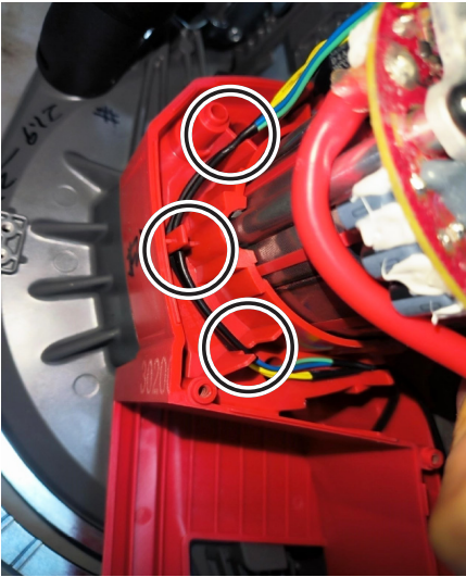
4) Press the colored wire into the housing traps and grooves around the stator.
