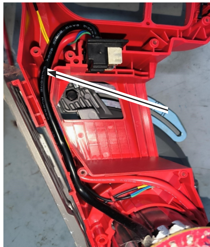
8) Press black wire into housing groove (on top of the red wire).
