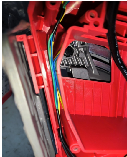
5) Press the colored wire into the housing traps and grooves as shown above.
