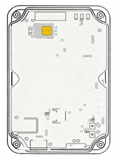
Figure_2 Remove the cover and insert SIM card
