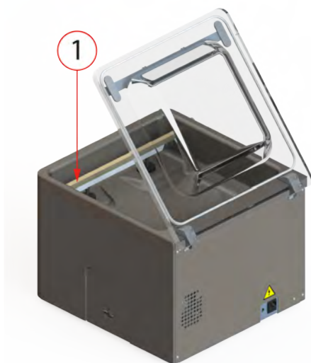
Figure 6: Removing the Sealing Bar
