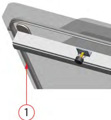
Figure 9: Replacing the Lid Gasket
