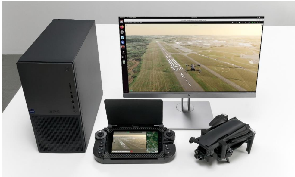
Figure 27: ANAFI UKR and Skycontroller UKR connected to a PC for the simulator
