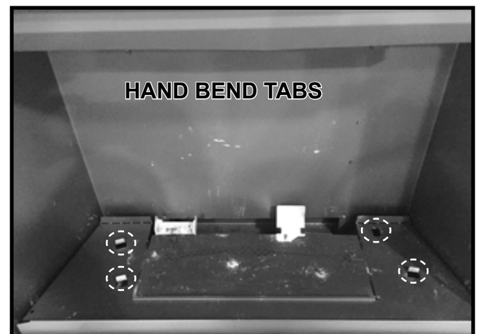
Figure 3. Hand Bend Tab Locations - QUARTZ36 Shown
