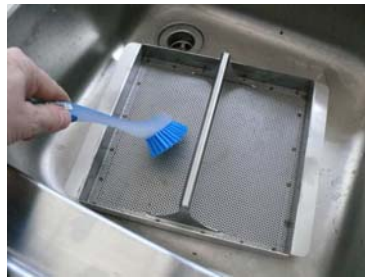
Clean the filter tank
