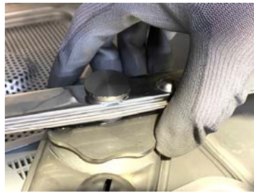
Daily disassemble the lower and upper wash arms by working on the „big“ ring nut, like in the picture.
