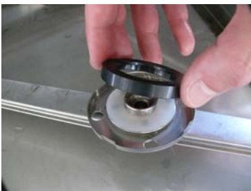
Control the wear washer cod.0201558 at the upper rinse arm is in his place.
