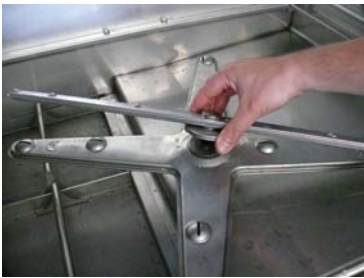
Screw the lower rinse arm
