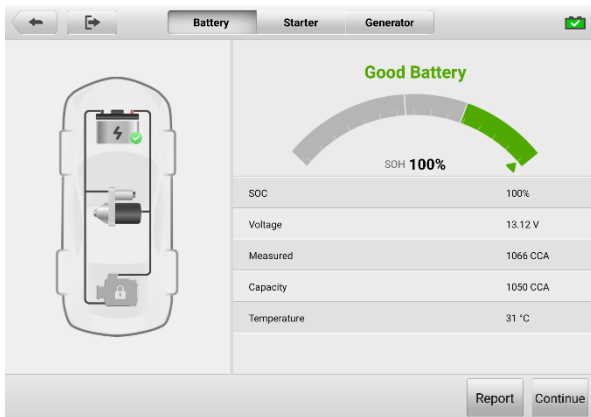
Figure 10-6 Battery Test Results
