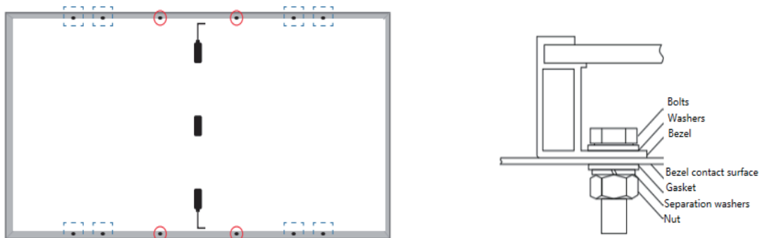
Figure 2 Schematic diagram of single-sided component mounting holes (The remaining component mounting holes are shown in the corresponding component layout)
