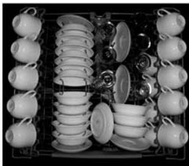
Top rack load pattern for 12 place setting according to the AHAM DW-1 Standards
