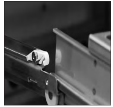
Fig. 7. Align the drawer with the drawer slide.
