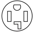
4-wire receptacle (14-30R)
