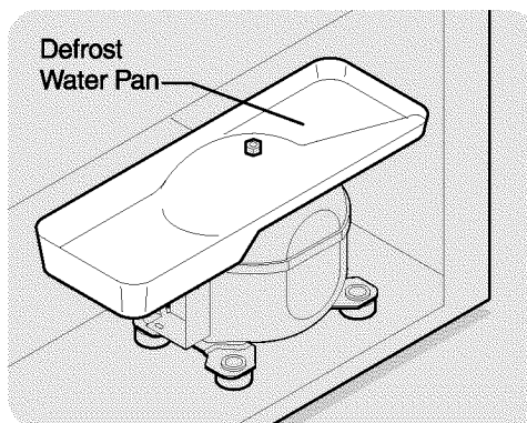
Nonremovable Defrost Water Pan (some models)
