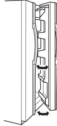
When the door is only partially open, it will automatically close. Beyond this stop the door will stay open.
