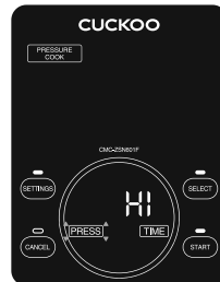
Before entering the preset setting mode (when selecting the PRESSURE COOK menu)
